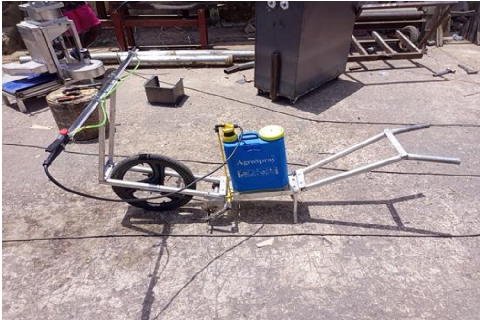
Figure 1: One wheeled, detachable four nozzles sprayer setup
