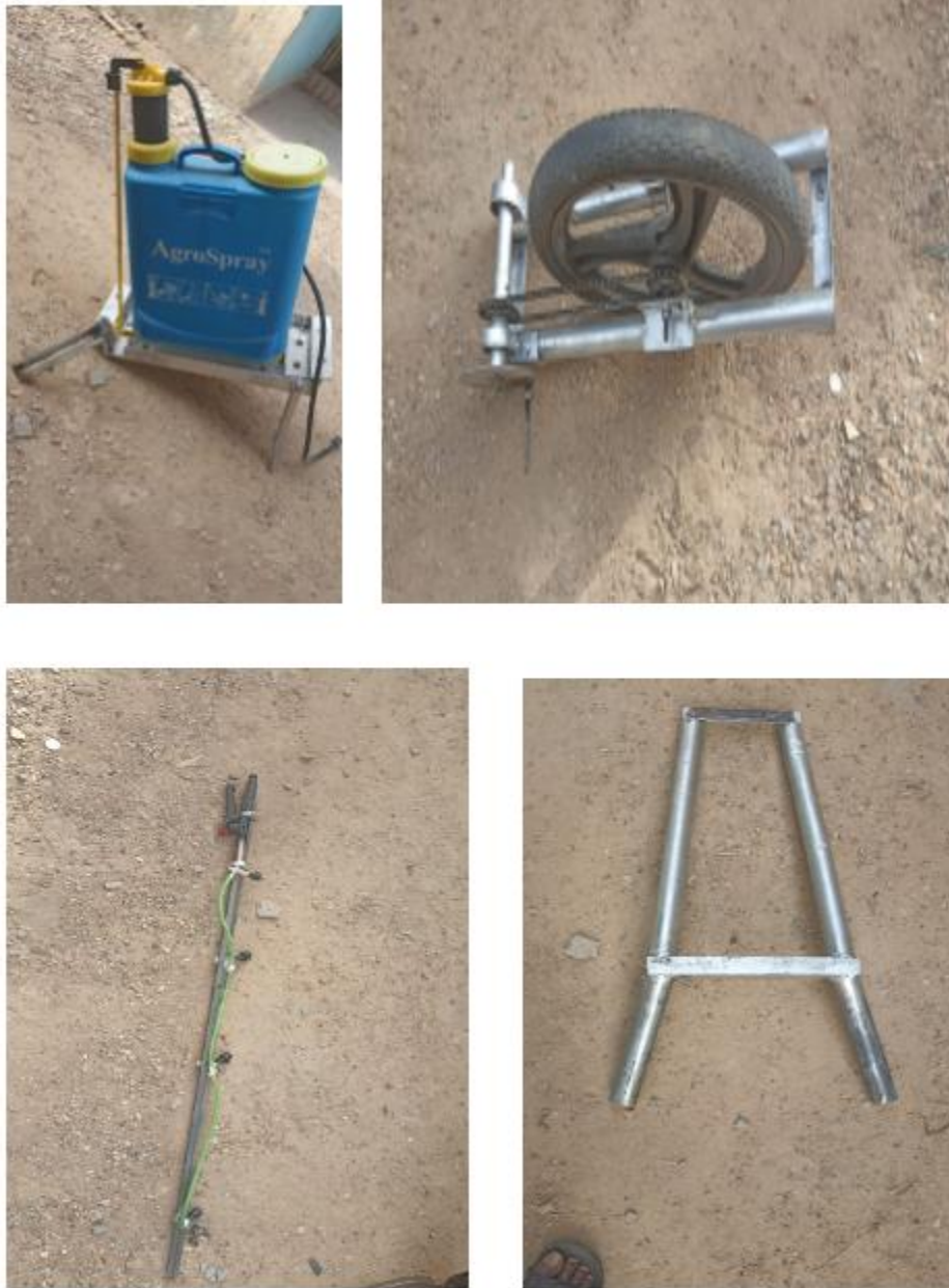
Figure 2: Components of the Designed Detachable Sprayer
