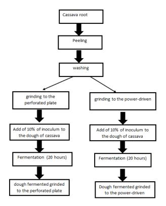
Fig. 5: Process for the preparation of fermented dough from grinders
